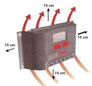
The regulator also generates heat during normal operation. The installation or assembly into another housing may not obstruct the rear vents necessary for cooling the device.
