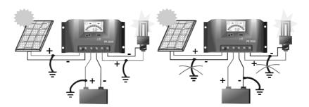
Observe that there is no common connection, e.g. across a ground connection, the minus module connections, battery minus and load minus. Non-observance can damage the regulator!
